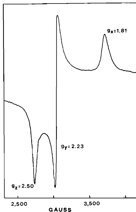
Fig. 1. Electron spin resonance spectrum at 95 K of a 3 \times 10^{-2} \text{ mol dm}^{-3} aerated solution of native cytochrome c (pH \approx 7 ) after irradiation with \lambda > 315 \text{ nm} light at room temperature. For specific conditions, see 'Materials and Methods'.
